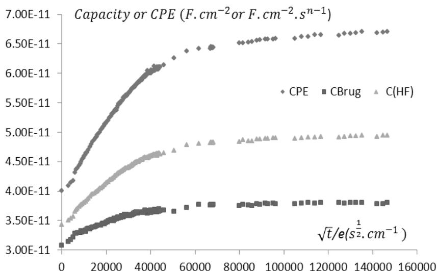
Figure 1: Evolution of the “film capacitance” with immersion time for an unstressed panel (thickness  $e$ ), aged at 30°C in NaCl solution.
