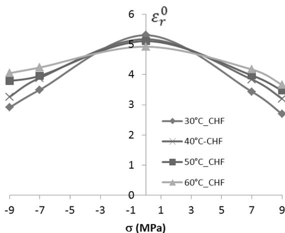
Fig. 2: Evolution of  $\varepsilon_r^0$  with  $\sigma$  using  $C_{HF}$ .
